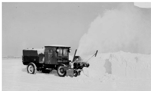
A snow plow truck with a blower in the 1920s [Chicago History Museum]
